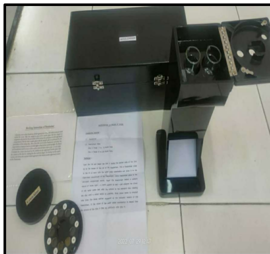
Hazen Scale with 2 discs (A-5 to 70, B-7 to 250)
