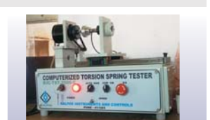
Computerized Torsion Spring Tester Capacity up to 10 NM
