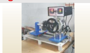
Manual Torsion Spring Tester Capacity up to 100 NM
