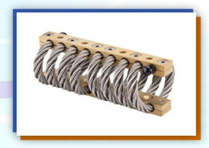
A Wire Rope Isolator is a robust and versatile vibration isolation device made from stainless-steel wire ropes that are looped and clamped between metal mounting bars. It is designed to absorb and reduce shock, vibration, and noise in various mechanical systems and equipment. These isolators are particularly valued for their durability, wide temperature tolerance, and ability to perform under extreme conditions
