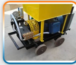
Hydro Testing Equipment
