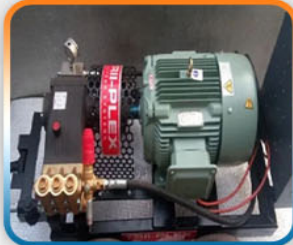
High Pressure Boiler Cleaning Pump
