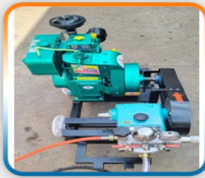
Diesel Engine Drive Hydro Test Pump
