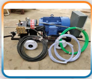
Boiler Tube Cleaning System
