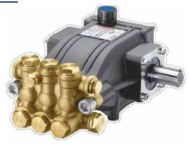
➤NHD150-C pumps can operate at a maximum pressure of 150 bar and with water temperatures up to 65°C (150F).
