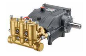
➤MXT pumps can operate at a maximum pressure of 200 bar, flow rates up to 100 lpm, and with water temperatures up to 65°C (149F).
