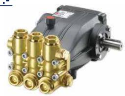
>XXT pumps can operate at a maximum pressure of 200 bar, flow rates up to 70 lpm, and water temperatures up to 65°C (149F).
