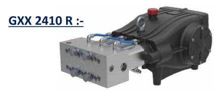
► GXX pumps can operate at a maximum pressure of 1000 bar and with water temperatures up to 65°C (149 F).
