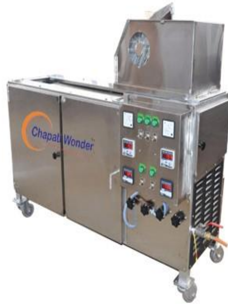
SEMI COMPACT CHAPATI MAKING MAKING MACHINE (100 TO 1500) PER HOUR
