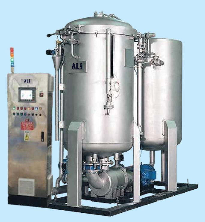
**Vertical Type HTHP Cone Dyeing Machine**
