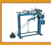
Direct Shear Test Apparatus
