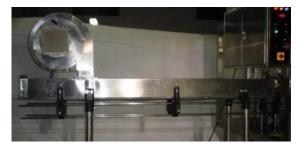
4. The machine will have 8 washing nozzles working under positive pump pressure of de-mineralized water. The machine does not include centrifugal pump for de-mineralized water.
