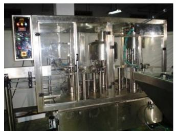
3. The bottles have to be loaded on the mouth of the Infeed Air conveyor. A blower is fitted on top of the frame of the Air conveyor. The air pushes the bottle further automatically and the bottles enter the Monoblock Rinsing, Filling & Capping machine. Total length of Infeed Air Conveyor is 5feet.
