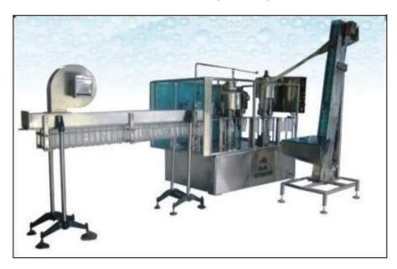
This is a mechanical machine with pneumatics for sturdiness, durability and maintenance free design. Certain internal mechanism of the machine, such as Cam, chain, and sprockets and rest frame structure etc. which will be internal & not exposed will be of Mild Steel cladded with Stainless Steel-304 sheet & product contact parts will be of Stainless Steel-316.
