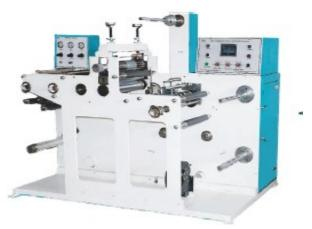
Designed for ROLL TO ROLL /SHEET ROTARY DIE CUTTING
