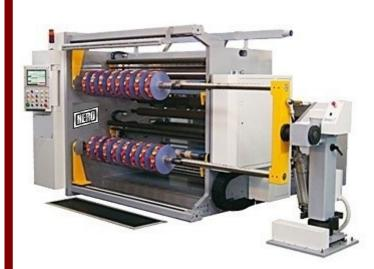
SHAFTLESS TYPE HEAVY DUTY UNWINDER WITH PNEUMATIC BRAKE AND WEB ALIGNMENT. A PNEUMATICALLY OPERATED SAFETY SHUTTER IS USED TO HOLD THE REWIND SHAFT WHILE REWINDING FOR CANTILEVER UNLOADING.
