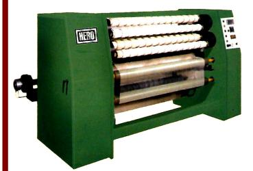
This compact and operator friendly machine is specially designed for high speed, Precision slitting and Rewinding of Self Adhesive paper, Crepe Paper, Polyester PVC Packaging, Laminated and BOPP Self Adhesive tapes.
