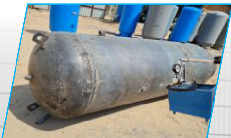
Hydro Testing upto 70 Kg/cm 2 Pressure
