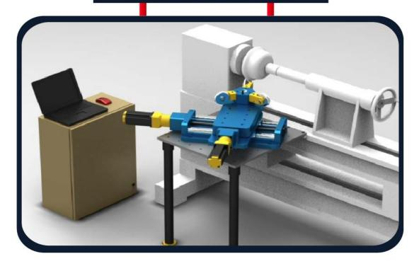
Currently there are two distinct types of machinery used for metal spinning: there are conventional hand spinning lathes which are commonly used as a rapid response solution for smaller quantity or specialized product runs. Secondly, there are computer numeric controlled (CNC) lathes, which are capable of producing thousands of precisely spun parts.
