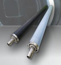
Fine bubble diffusers produce a plethora of very small air bubbles which rise slowly from the floor of a wastewater treatment plant or sewage treatment plant aeration tank and provide substantial and efficient mass transfer of oxygen to the water. The oxygen, combined with the food source, sewage, allows the bacteria to produce enzymes which help break down the waste so that it can settle in the secondary clarifiers or be filtered by membranes.
