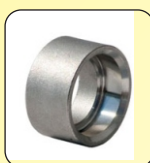
Female Half Coupling (Threaded/Socket Weld) - Alloys - T304 and T316 Stainless Steel, Carbon Steel, Malleable Iron, Brass - Sizes - 1/4" thru 4" - Class - 150#, 3000#
