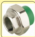
Female Union (Threaded/Socket Weld) - Alloys - T304 and T316 Stainless Steel, Carbon Steel, Malleable Iron, Brass - Sizes - 1/4" thru 4" - Class - 125#, 150#, 3000# (Carbon Steel Only)
