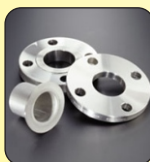
C Stub with Floating Flange Alloys - T304 and T316 Stainless Steel Sizes - 1 1/2" thru 10" Schedule - 10
