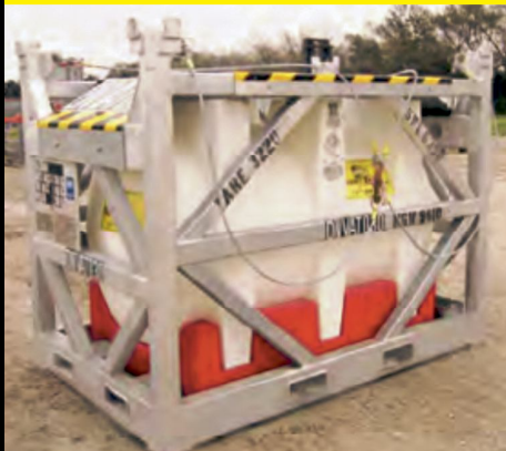
550 GALLON ACID TANK (Poly IBC)
