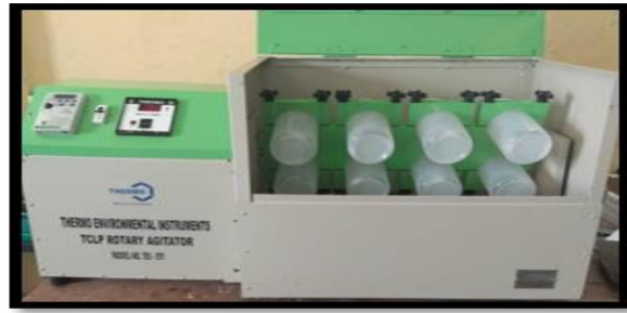
TCLP ROATY AGITATOR THERMO MODEL TEI-551 (FOR SOLIDS AND WASTES - TOXICITY CHARACTERISTIC LEACHING PROCEDURE)
