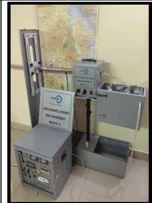
DIOXINS & FURANS STACK MONITORING KIT THERMO MODEL TEI - 141
