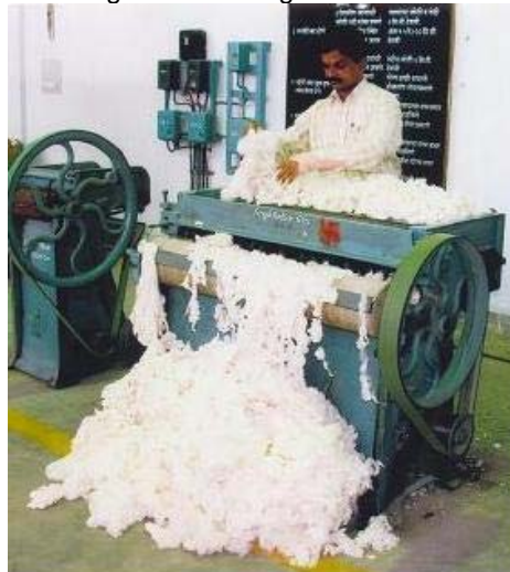
Figure 3.3.1 Single Roller Gin
