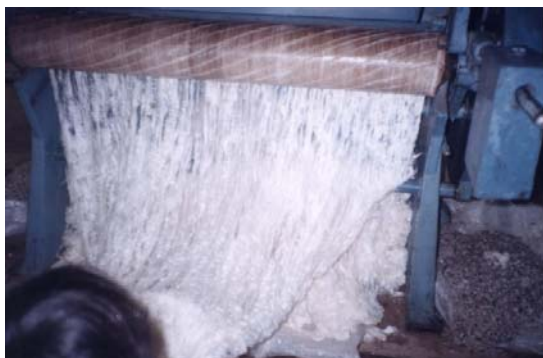
Figure 3.3.3 (a) Double Roller Gin machine
