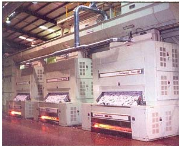
Figure 3.2 Saw Gin stands in ginnery in USA
