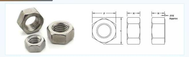
A six-sided internally threaded fastener with metric thread / inch Thread pitch. 16 millimeter nuts and smaller are chamfered on the top and the bearing surface. Larger nuts may be double chamfered, or have a washer face on one side and a chamfered surface on the opposite side.
