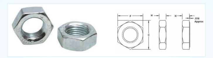
A six-sided internally threaded fastener which is thinner than the thickness of a finished hex nut. Used in combination with a finished hex nut to keep the nut from loosening.
