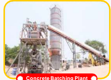
Concrete Batching Plant
