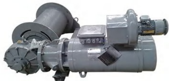
PC Hoist Mechanism PC 起升机构
