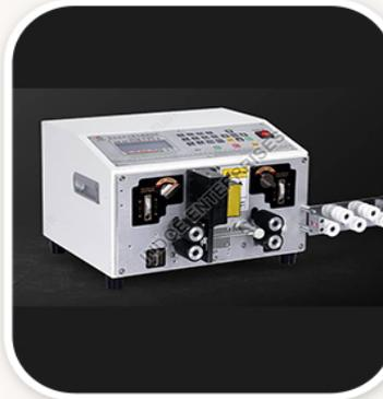
**IE-220 High Speed Wire Cutting & Stripping Machine**
