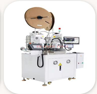
**Double End Wire Cutting, Stripping & Crimping Machine**
