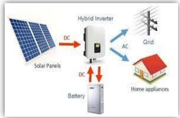
Hybrid (Solar + Battery + Grid)
