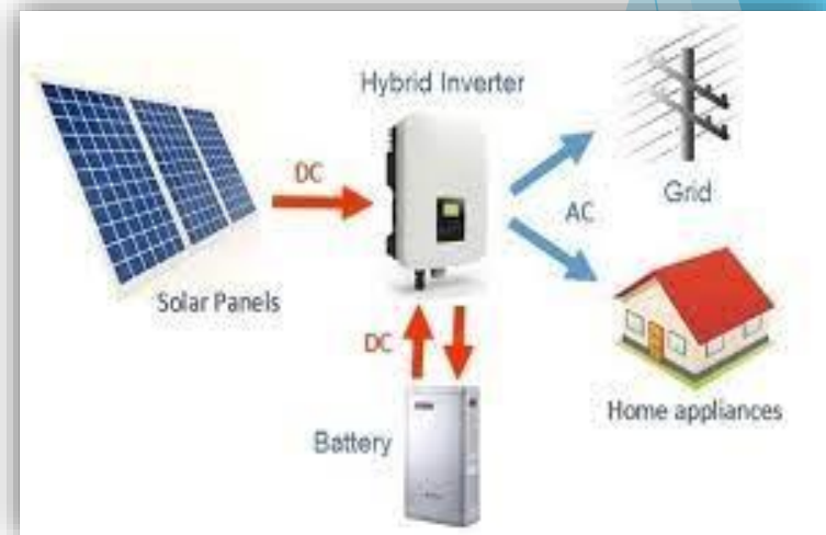
Hybrid (Solar + Battery + Grid)
