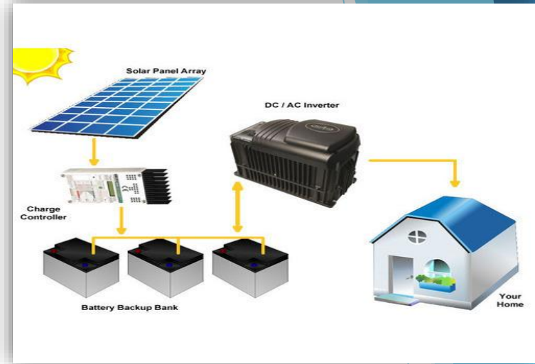
Off Grid (Solar + Battery Storage)
