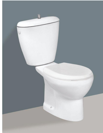
8002-Italian Set P/S Trap S Trap : 225mm (9") Size : 625x430x780mm
