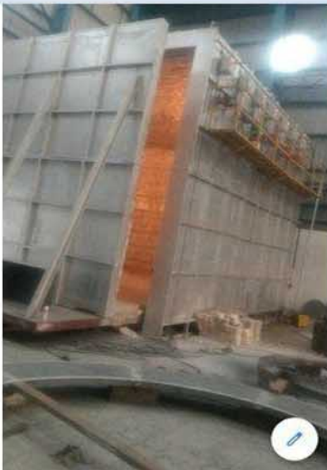
Stress Relieving Furnace 50 Ton
