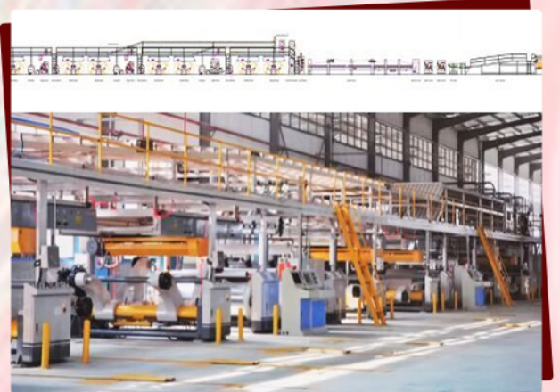
Automatic Corrugated Carton Board Box Making Plant
