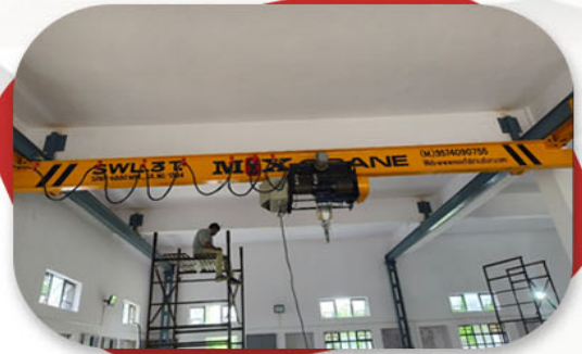
SINGLE GIRDER UNDERSLUNG EOT CRANE
