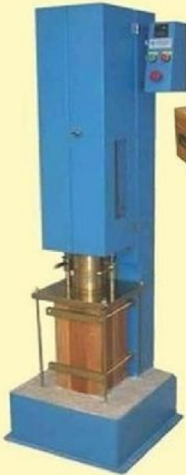
Automatic Bitumen Compactor
