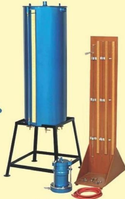
Soil Permeability Test
