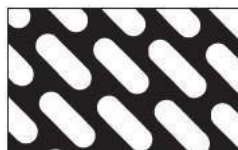
Round ended slotted side staggered at 45 degrees
