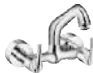
F2012511 Sink mixer (wall mounted) with 185 mm (7.5") long swivel spout, connecting legs and wall flanges ₹ 5320
