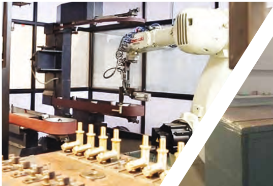
▲ Robotic Surface Grinding - Faucet
