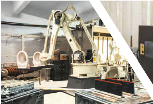
▲ Robotic Glazing - Sanitaryware
